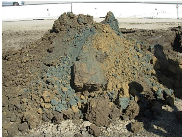
Photo 6 – Stained (bluish green) stockpiled soil.
