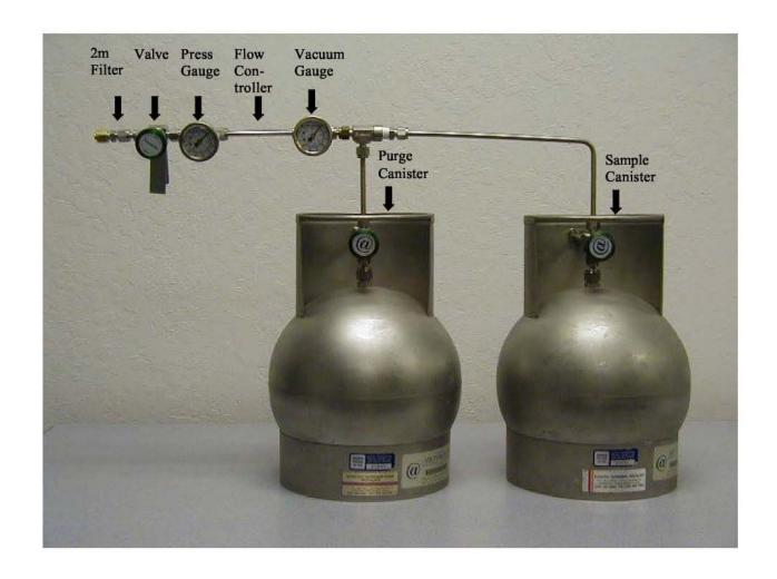
Figure 4 Typical Soil Gas Sampling Manifold 8410 Amelia Street Oakland, California
