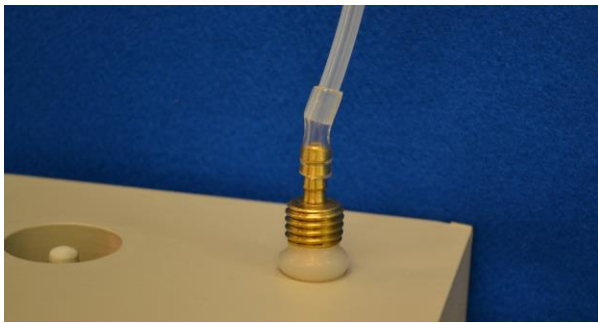
Figure 5. VAPOR PIN® sample connection
