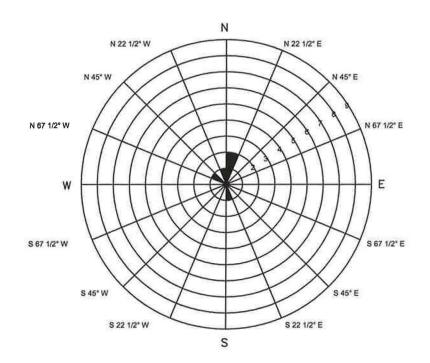
Rose diagram developed by evaluating the groundwater gradient direction from the quarterly monitoring data. Each circle on the rose diagram represents the number of monitoring events that the gradient plotted in that 22 1/2 degree sector.
