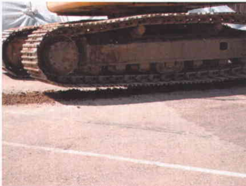
Cleaning soil off of the excavator's treads
