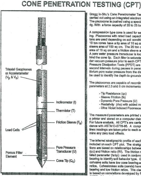
Gregg In-Situ's Cone Penetrometer Tests (CPT) are carried out using an integrated electronic piezocone. The piezocone is pushed using a specially designed CPT rig. With a force capacity of 20 to 25 tons.
