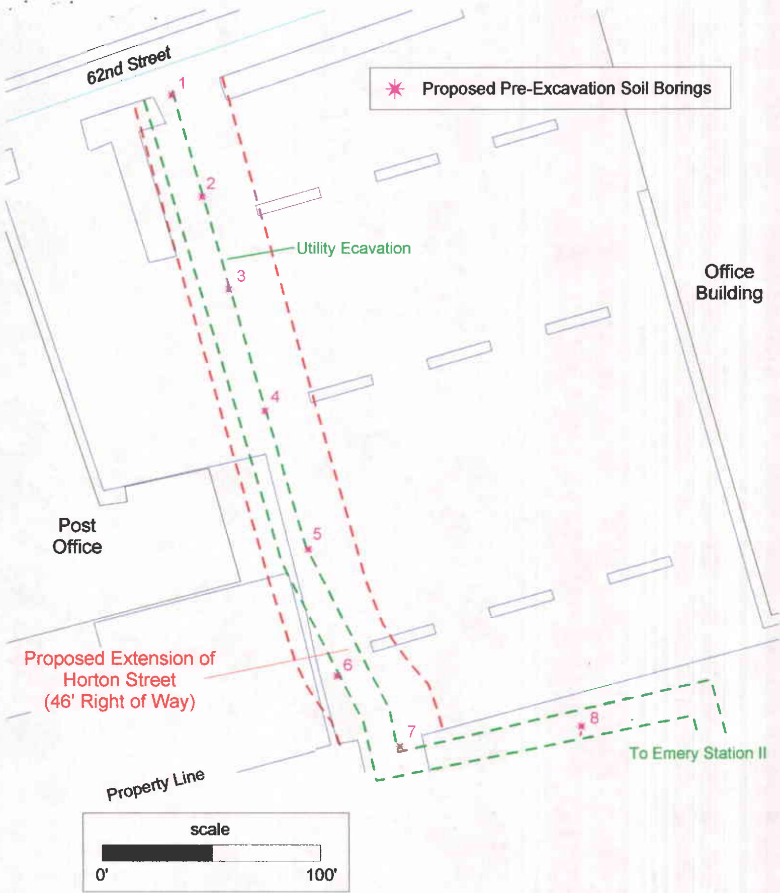
Figure 4: Location of Proposed Pre-Excavation Soil Borings
