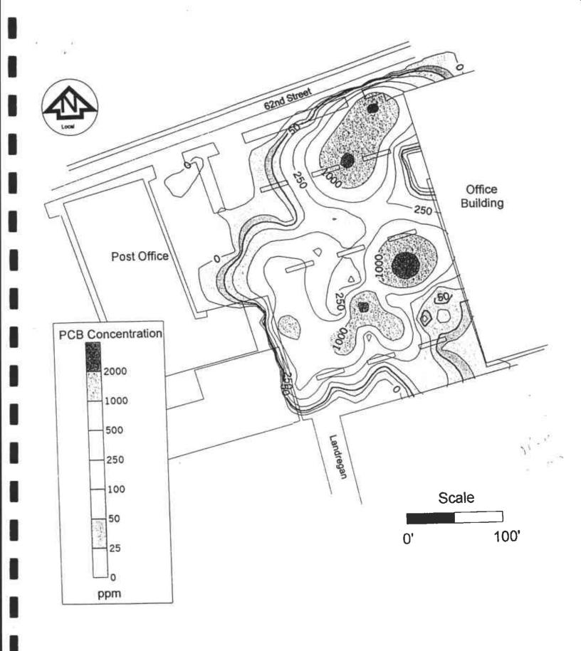
Figure 2: Contour Map of PCB Concentrations (ppm) at 0.5' Depth
