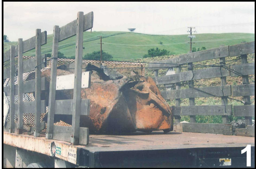
UST Loaded on the Truck April 15, 2004
