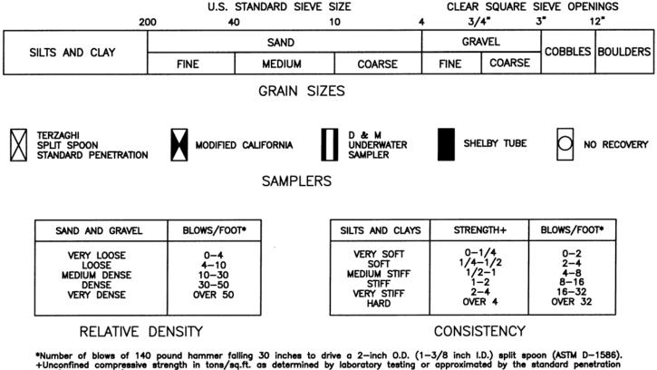
\*Number of blows of 140 pound hammer falling 30 inches to drive a 2—inch 0.D. (1—3/8 inch I.D.) split spoon (ASTM D—1586). +Unconfined compressive strength in tons/sq.ft. as determined by laboratory testing or approximated by the standard penetration test (ASTM D—1586), pocket penetrometer, torvane, or visual observation.
