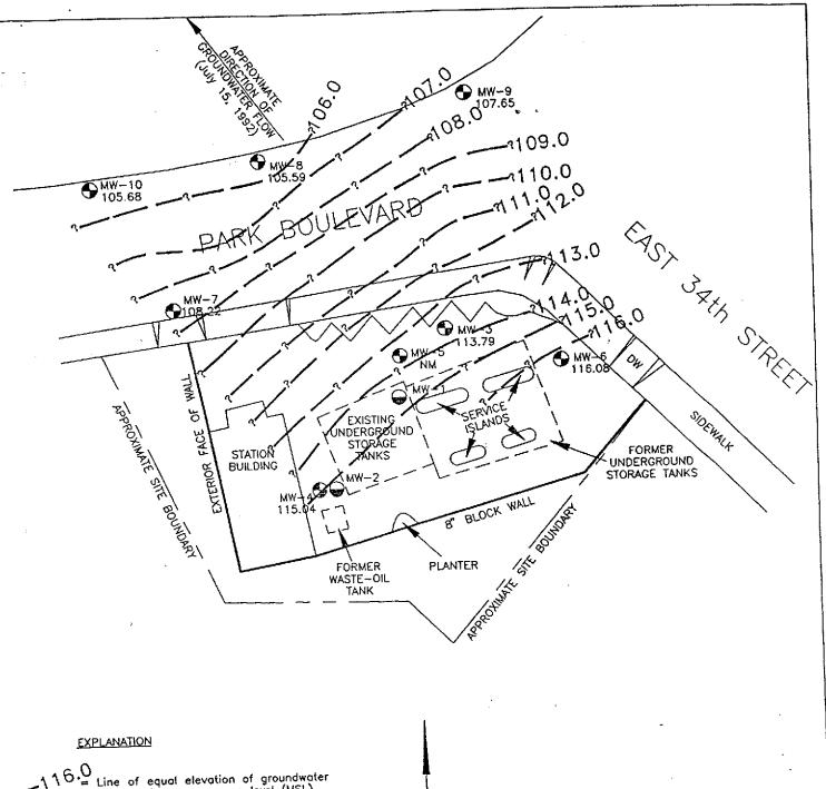
16.9 Line of equal elevation of groundwater in feet above mean sea level (MSL)
