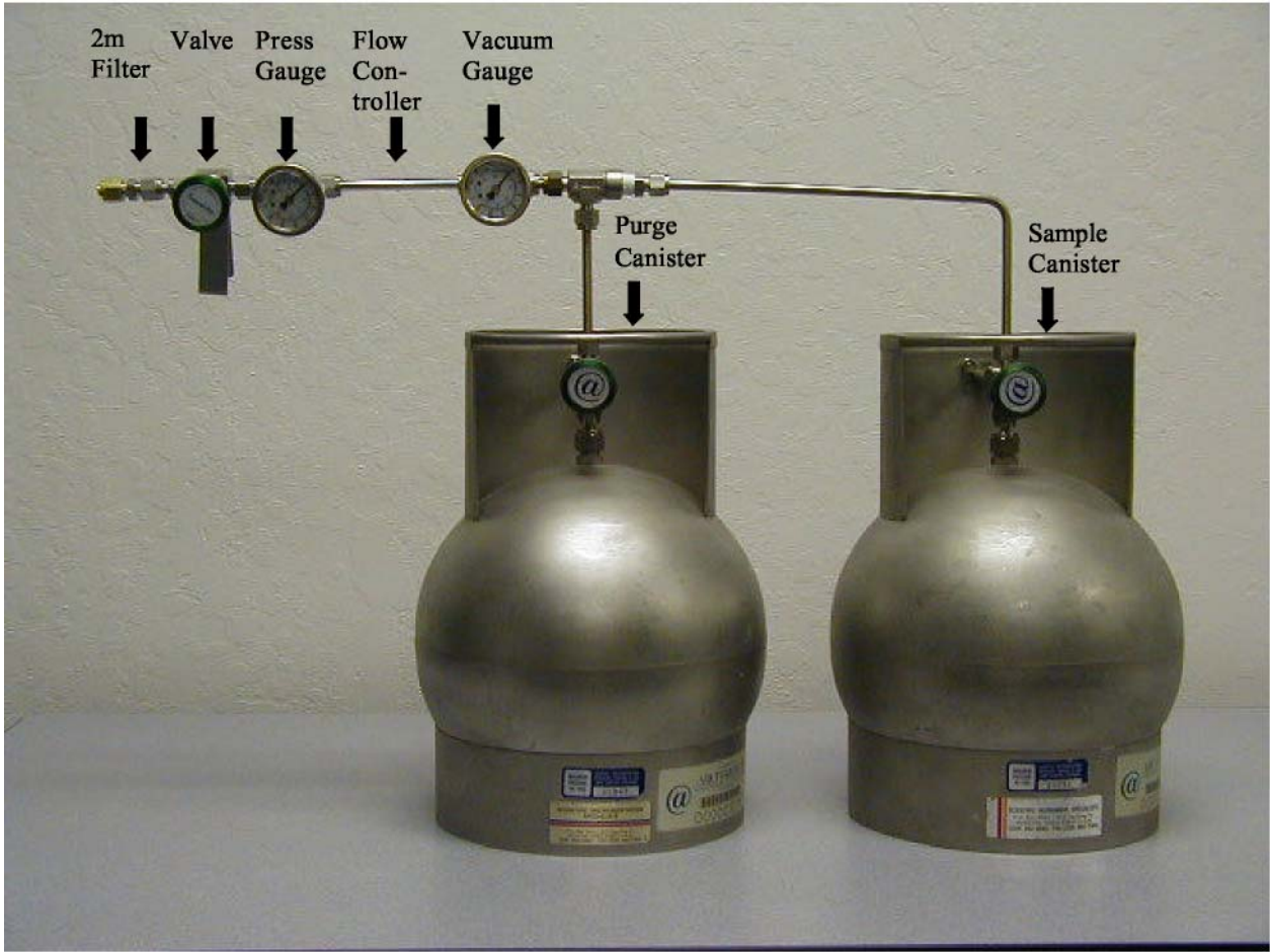
Figure 5 - Typical Soil Gas Sampling Manifold
