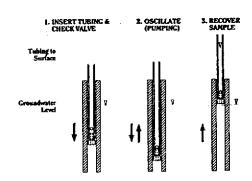
Groundwater Sampling with a Tubing and Bottom Check Valve
