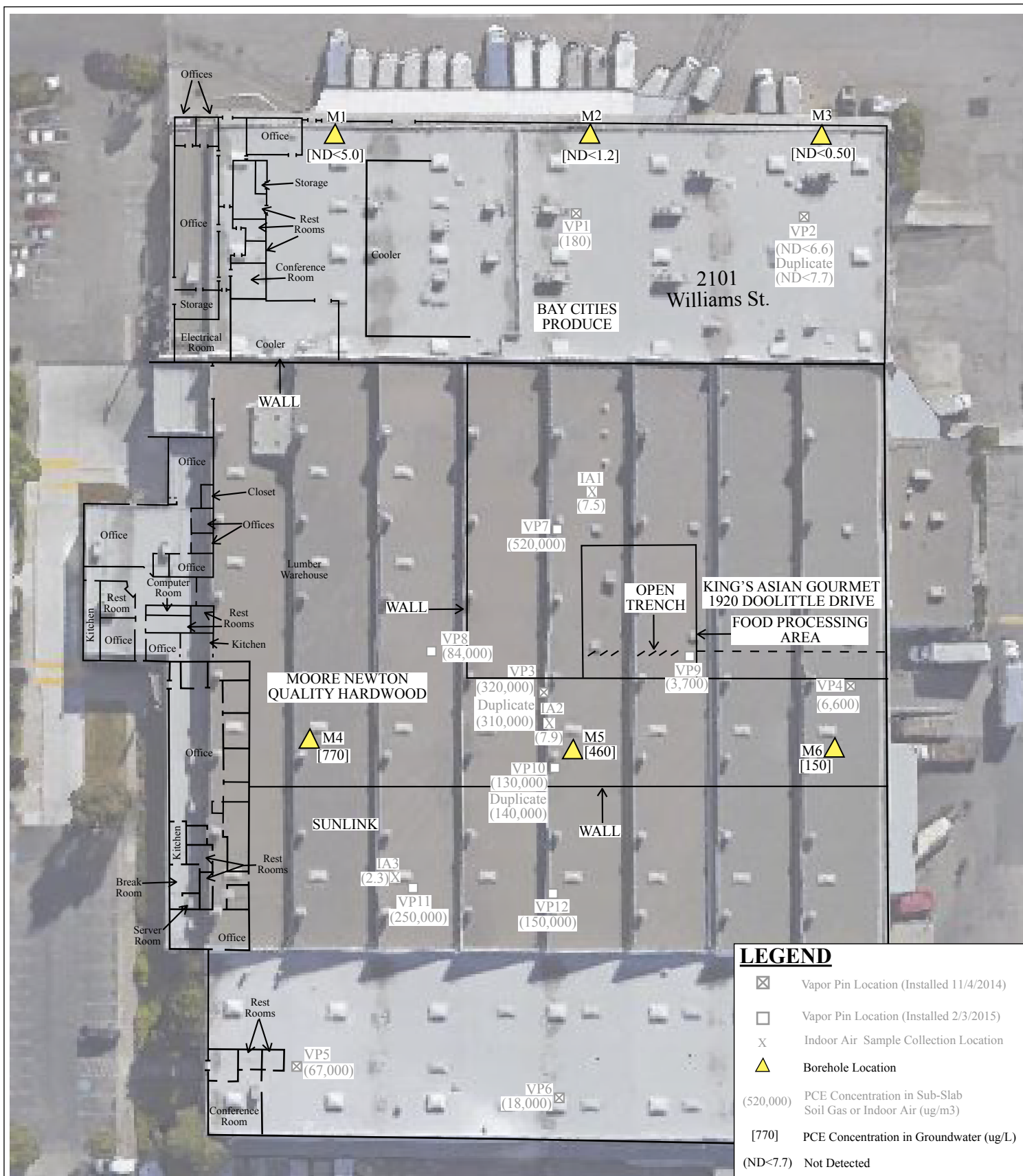
Figure 2 Site Plan Aerial Photograph Detail Showing PCE Concentrations in Groundwater at 20-Foot Depth 2101 Williams Street San Leandro, California
