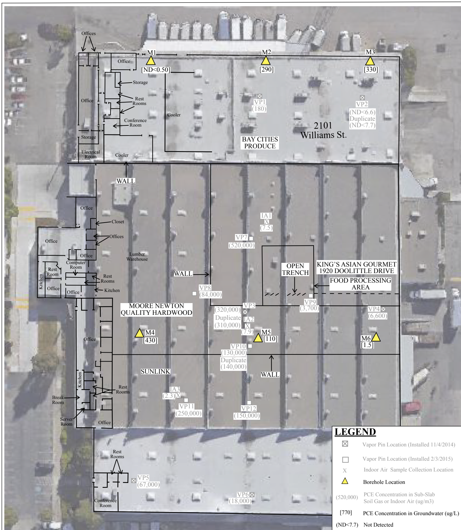
Figure 3 Site Plan Aerial Photograph Detail Showing PCE Concentrations in Groundwater at 30 to 35-Foot Depth 2101 Williams Street San Leandro, California
