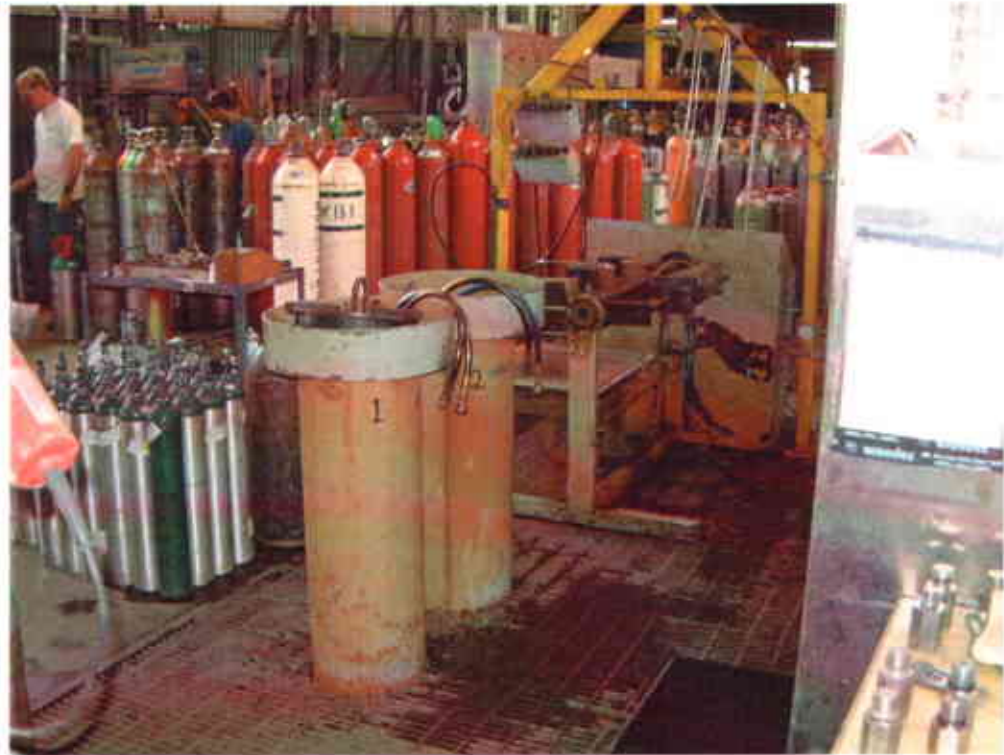
Photo #7: Elevated hydrostatic cylinder testing apparatus over wastewater sump in southwest end of Building One. Bead blast cylinder paint remover in center background, against far wall.
