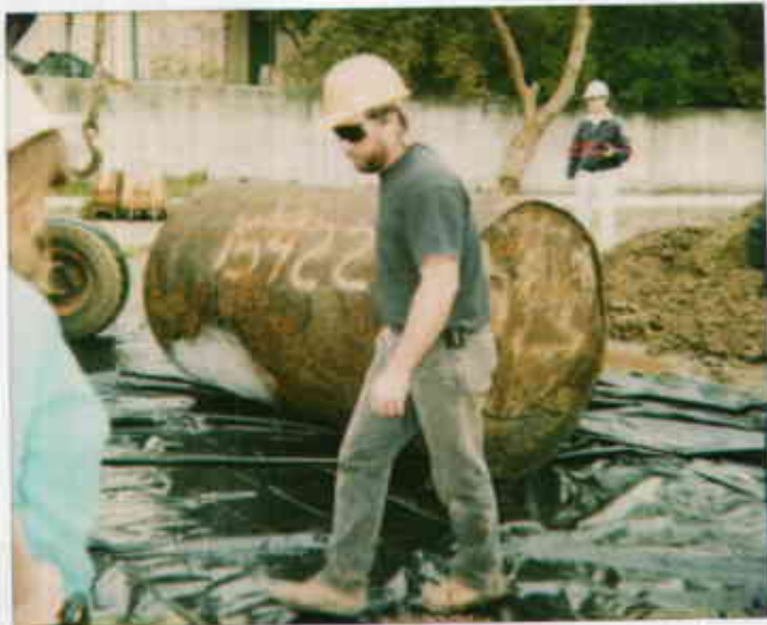
Shell Oil 7416314507-2 3/7/95 9750 Golf Links #15 - Oakland 8453 8461 500 gal w.o. 157 - Numerous small holes - pitting & rust.
