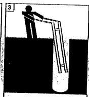
By pulling both the release tool and removal tool, remove SAFE-T-SHORE from trench.
