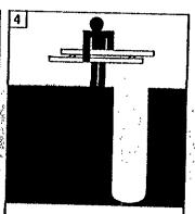
Remove tools from shore and fold SAFE-T-SHORE flat to be carried to next installation point.
