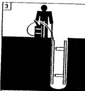
With free hand, turn ¼ turn valve on pump to closed position. Pump shore to a minimum pressure of 750 pounds per square inch (psi) as shown on pump gauge. Higher pressures can be used when needed Remove hook from handle.
