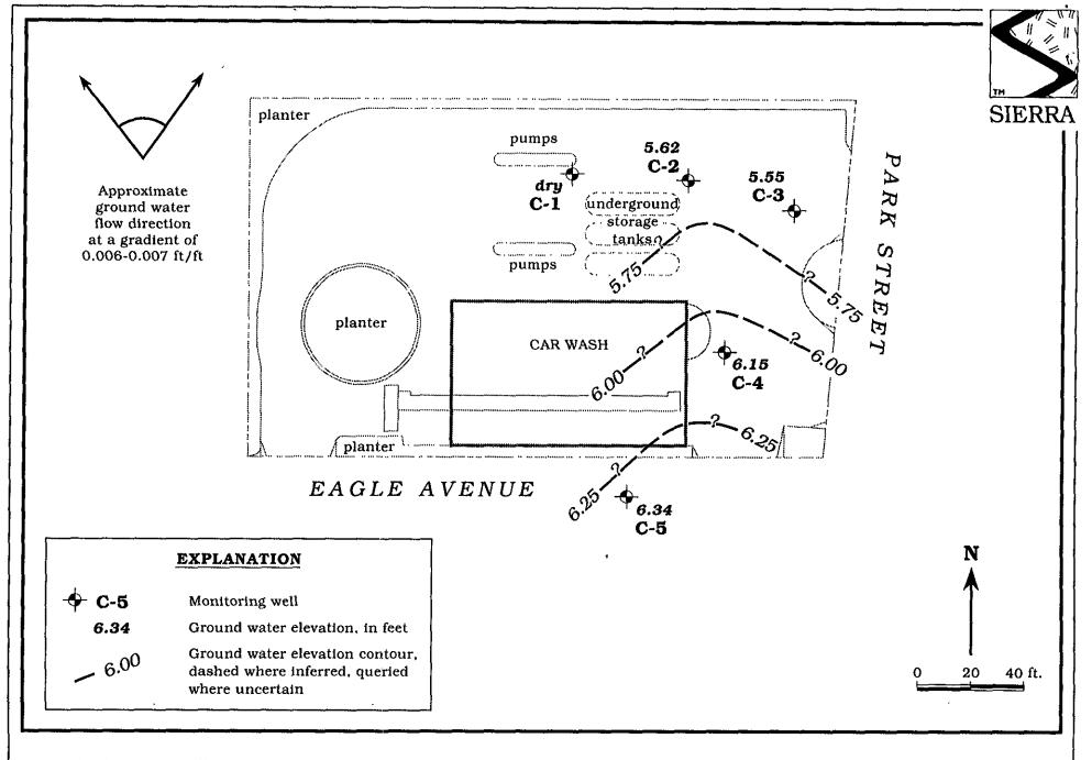
Figure 1. Monitoring Well Locations and Ground Water Elevation Contour Map - August 25, 1994 - Chevron Service Station #9-4463, 1801 Park Street, Alameda, California
