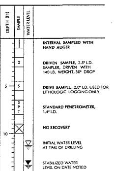
SOIL CONDITIONS INDICATED BY BORING LOGS APPLY ONLY AT THE LOCATION OF THE PARTICULAR BORING AND AT THE TIME OF DRILLING, SUBSURFACE CONDITIONS MAY DIFFER AT OTHER LOCATIONS AND MAY CHANGE AT THE BORING LOCATION WITH THE PASSAGE OF TIME. DATA PRESENTED IN THE LOGS REPRESENT A SIMPLIFICATION OF THE ACTUAL CONDITIONS ENCOUNTERED, SOIL CONDITIONS INDICATED BETWEEN SAMPLE INTERVALS ARE INFERRED.
