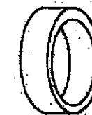
5.0 O.D. X 4.0 I.D. COMPRESSION SEAL
