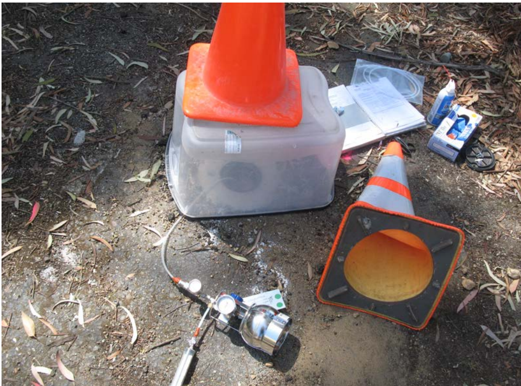
Photo 22: Soil gas sampling equipment and leak detection shroud (plastic container) at location SG-5.
