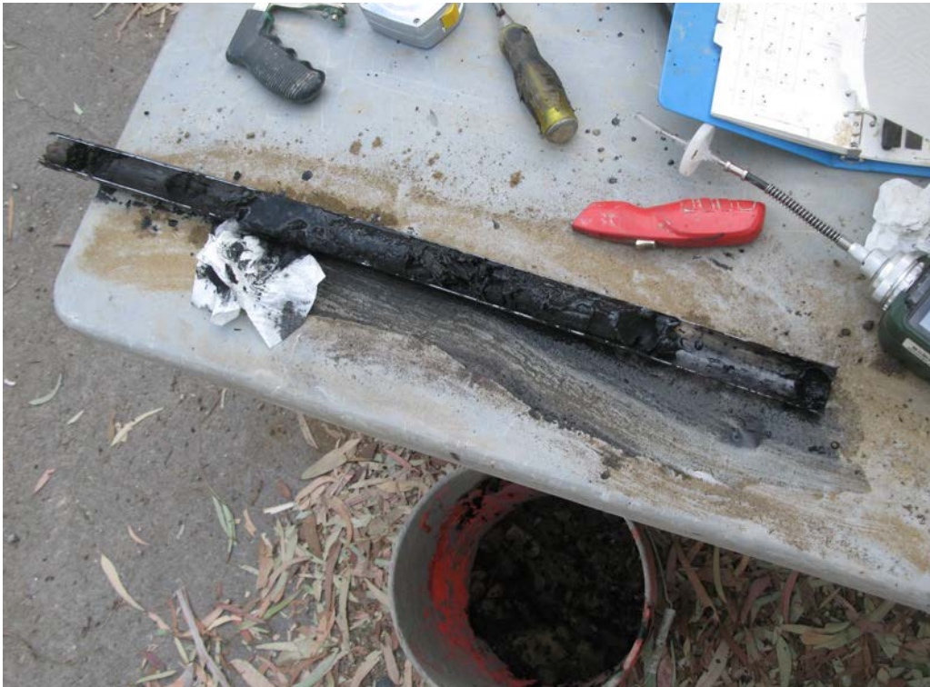
Photo 19: Black-colored soil and groundwater observed within the saturated zone at SG-5.
