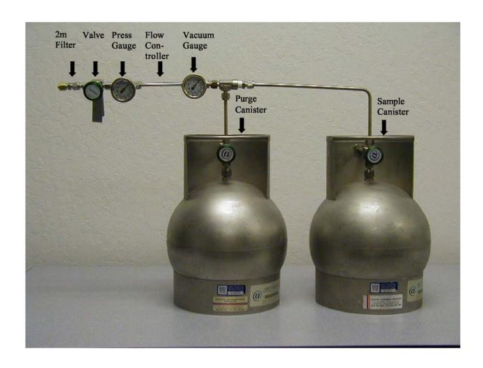
Figure 7. Typical Soil Gas Sample Collection Manifold
