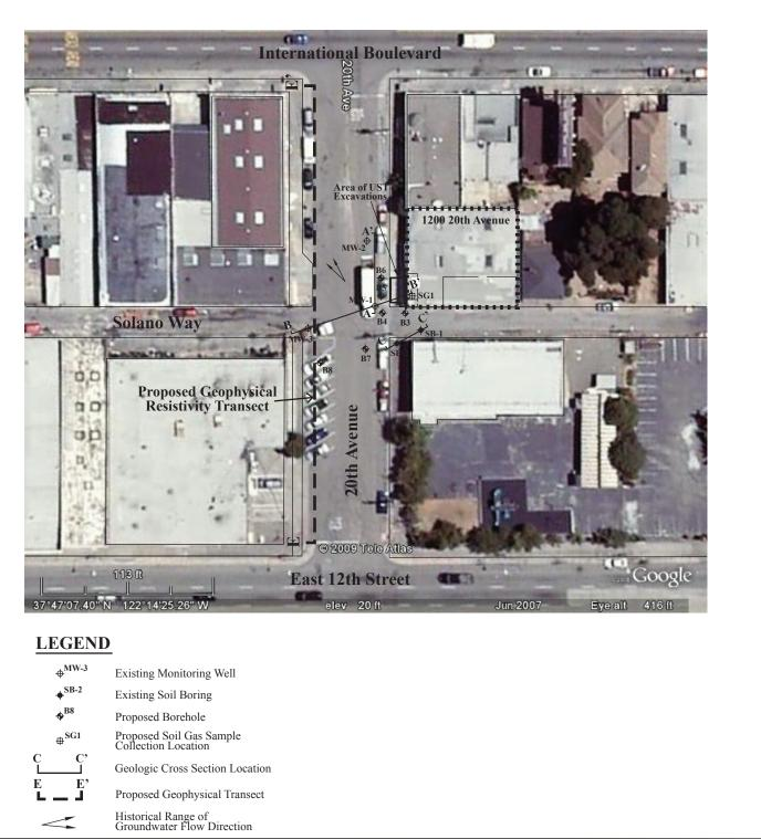
Figure 2 Site Vicinity Map Showing Existing and Proposed Drilling Locations, and Locations of Cross Sections and Proposed Resistivity Transect William Wurzbach Company 1200 20th Avenue Oakland, California
