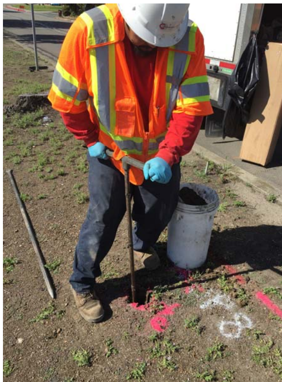
Plate 4. Hand Augering DP-8 to 5 Feet bgs
