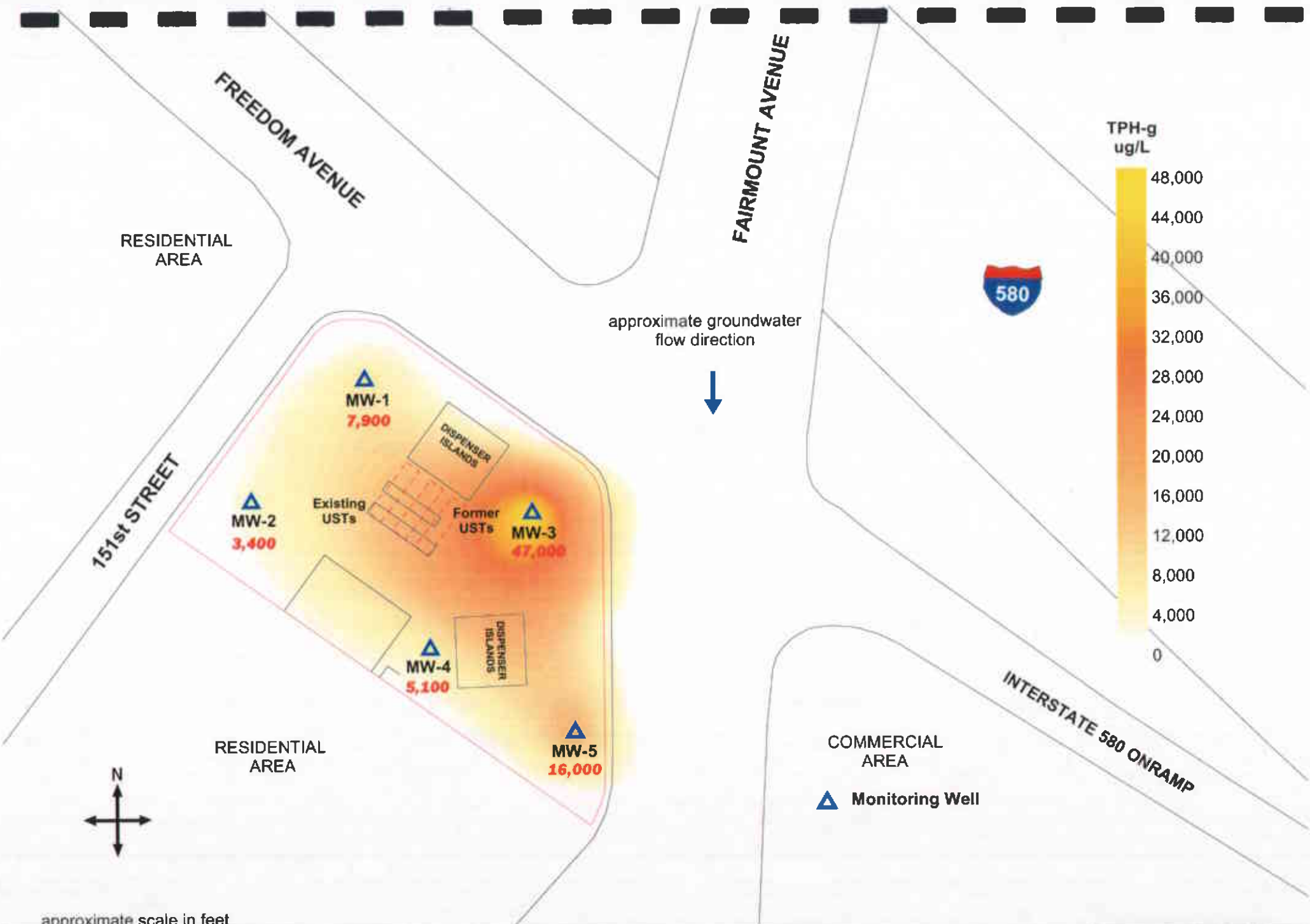
Figure 4: Contour map of TPH-g concentrations in groundwater. November 8, 2002.
