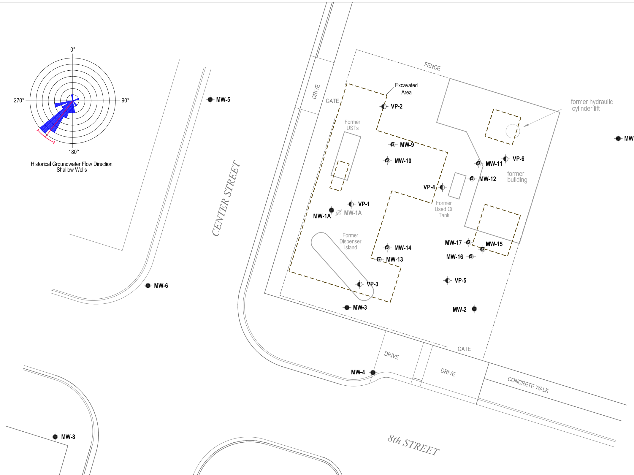
FIGURE 2 SITE PLAN with WELLS and VAPOR PROBE LOCATIONS FORMER CHEVRON SERVICE STATION 20-6145 800 CENTER STREET Oakland, California
