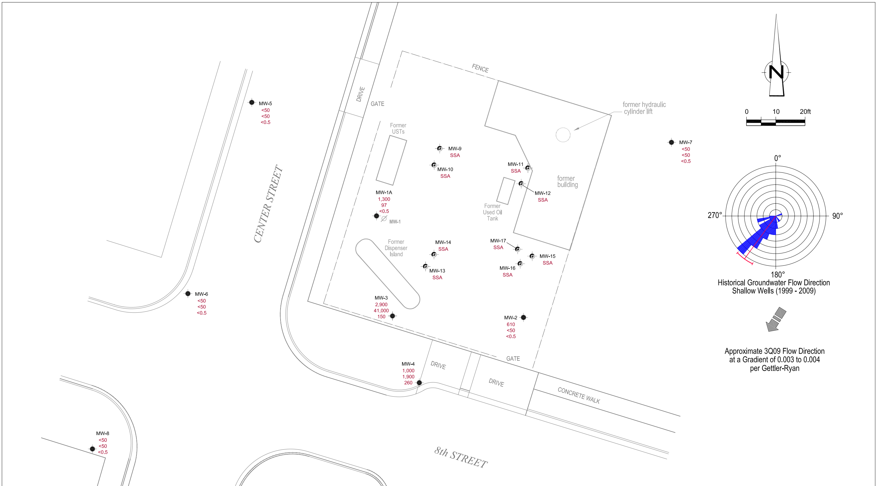
FIGURE 2 HYDROCARBON CONCENTRATIONS IN GROUNDWATER FORMER CHEVRON SERVICE STATION 20-6145 800 CENTER STREET Oakland, California August 7, 2009
