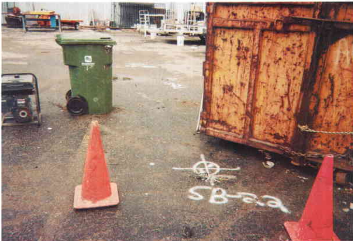
Photo 1: Soil borings along western edge of gasoline-affected soil (SB-22 in foreground and SB-21 and SB-20 in middle background).
