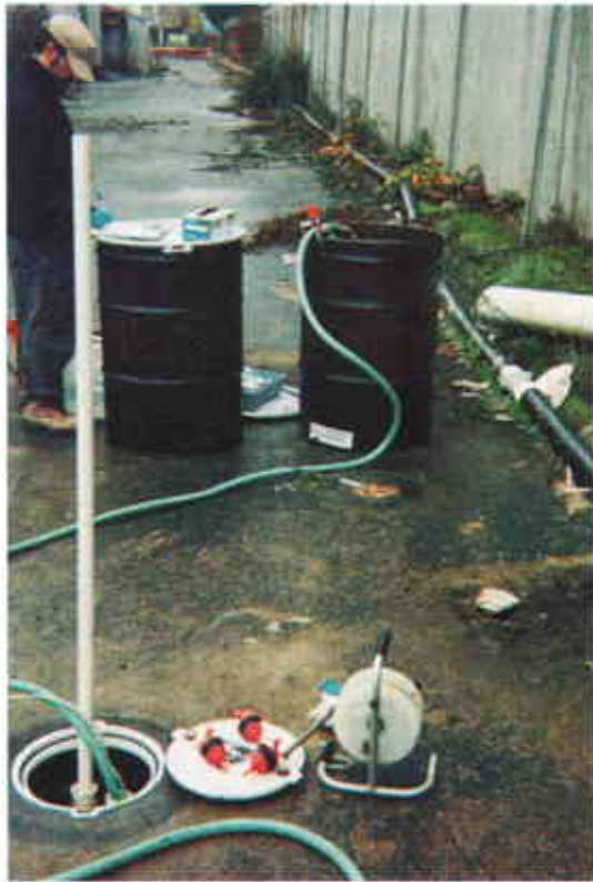
Photo 14: Sampling equipment used during collection of groundwater samples from nested wells.
