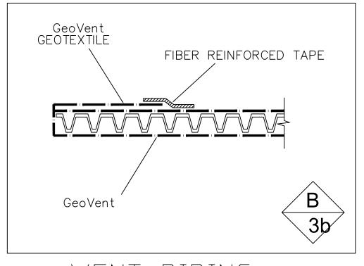
VENT PIPING TERMINATION DETAIL
