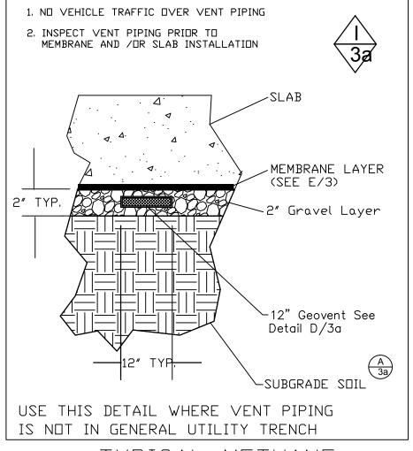
TYPICAL METHANE PIPE TRENCH DETAIL
