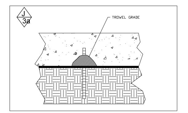
RE-BAR PENETRATION REPAIR DETAIL
