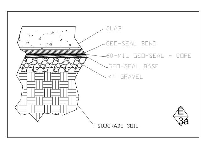
MEMBRANE LAYERING FOR Geo-Seal
