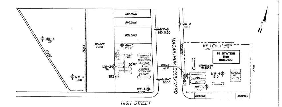
MW-7 + 76 Station Monitoring Well with Dissolved-Phase MTBE Concentration (μg/1)
