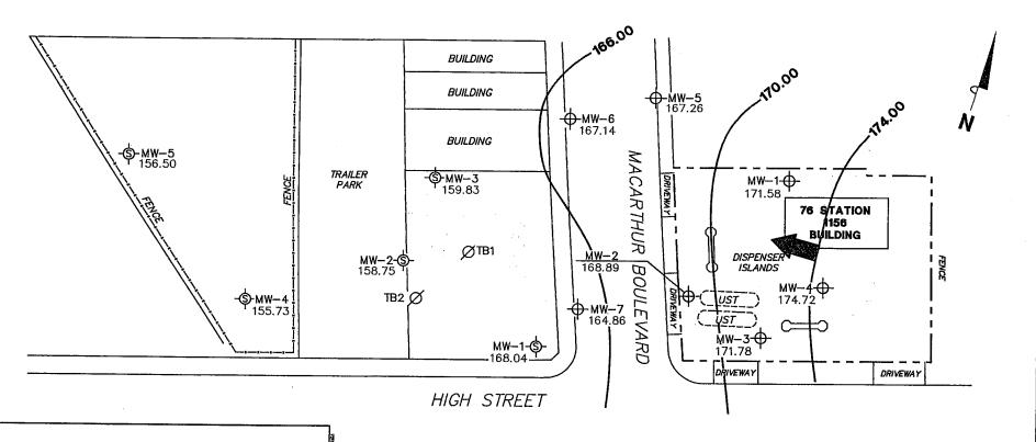
MW-7 + 76 Station Monitoring Well with Groundwater Elevation (feet)
