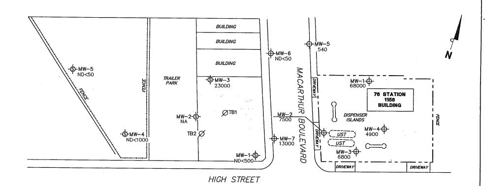
MW-7 + 76 Station Monitoring Well with Dissolved—Phase TPH—G Concentration (μg/I)
