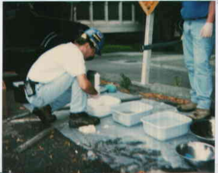
2740 Broadway, Oakland 08/05/99 08916310210-02 0125 5073 COPIES & ENLARGEMENTS CALL 800-421-1030 ESE consultants collecting soil samples from SB-1E & SB-2E. - Juliet Shinn
