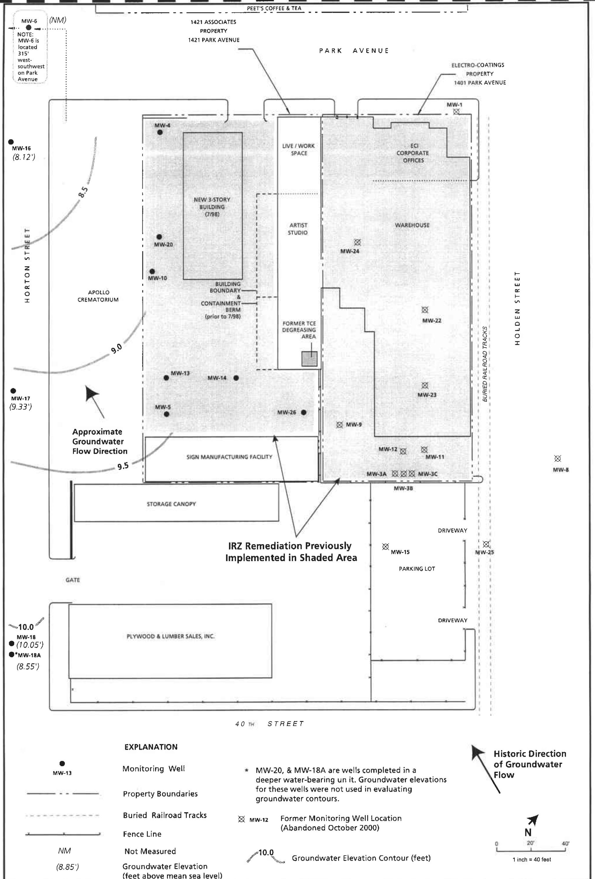
**SITE PLAN WITH GROUNDWATER ELEVATION CONTOURS (FEBRUARY 2001)**
