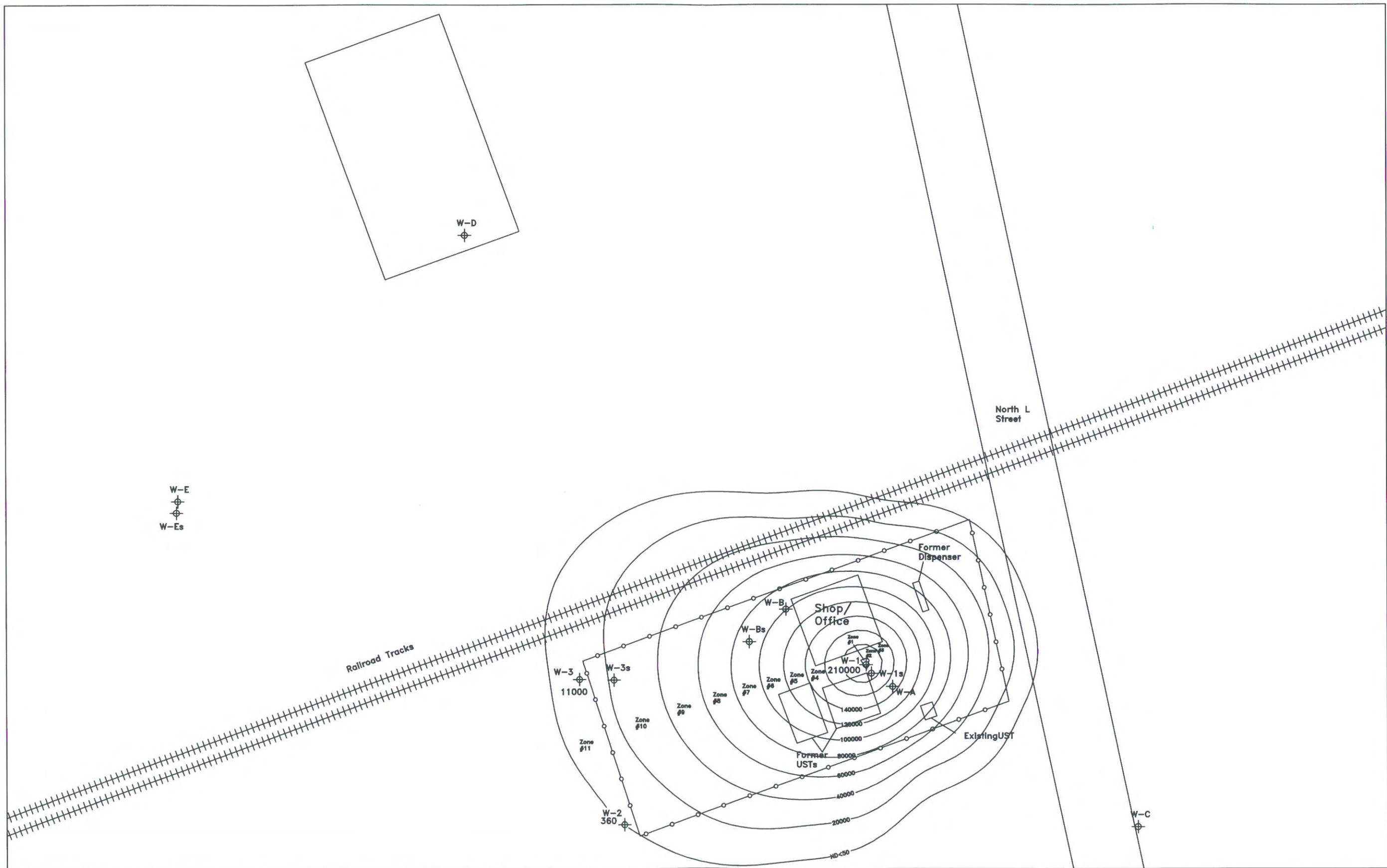
Fig 6: Shallow Well 1988 Gasoline Concentrations
