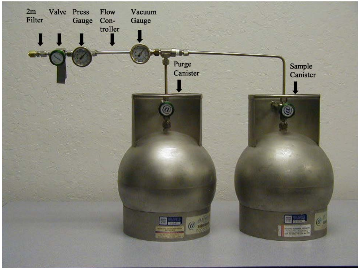
Figure 8. Typical Soil Gas Sample Collection Manifold
