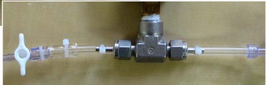
Fig 1: Attach syringe & vacuum gauge to soil gas probe tubing using 2-way & 3-way valves. Be sure to zip tie the connections.
