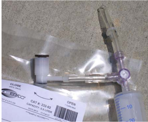
Fig 2: Connect tedlar to the side port of the 3-way valve and fill bag with 300-450 cc vapor sample.
