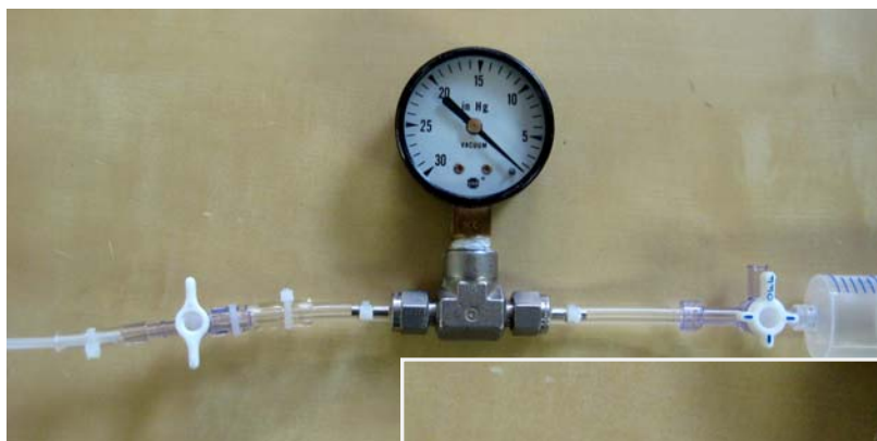
Fig 1: Attach syringe & vacuum gauge to soil gas probe tubing using 2-way & 3-way valves. Be sure to zip tie the connections.
