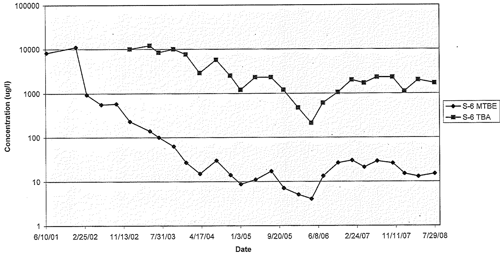
Graph 2 MTBE and TBA Concentrations Well S-6 Shell-branded Service Station 3790 Hopyard Road Pleasanton, California
