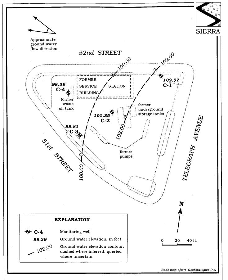
Figure 2. Monitoring Well Location and Ground Water Elevation Contour Map - September 16, 1992 - Former Chevron Service Station #9-3864, 5101 Telegraph Avenue, Oakland, California
