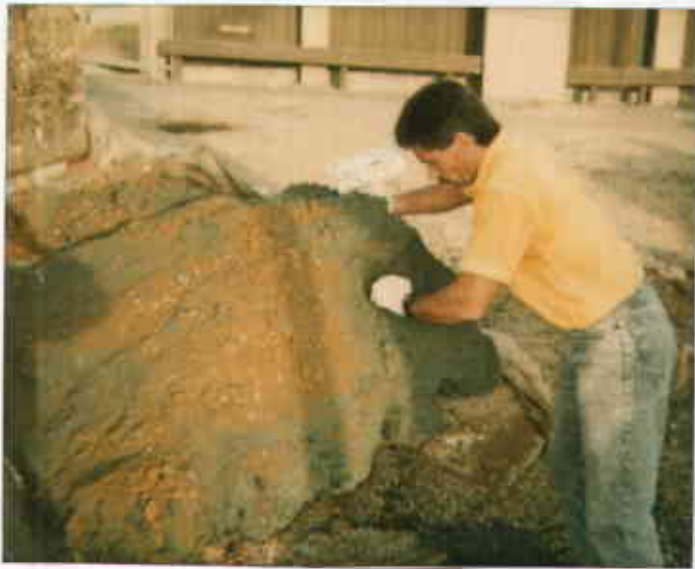
Sampling from material along east wall of excavation
