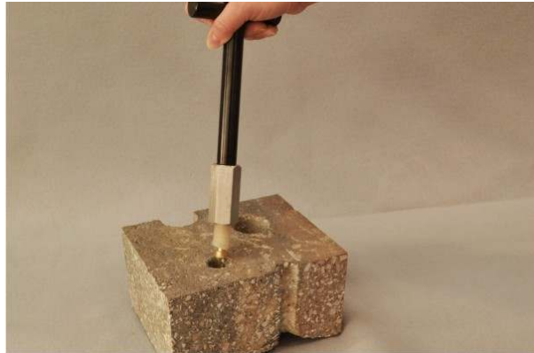
Figure 8. Extracted Vapor Pin™.
