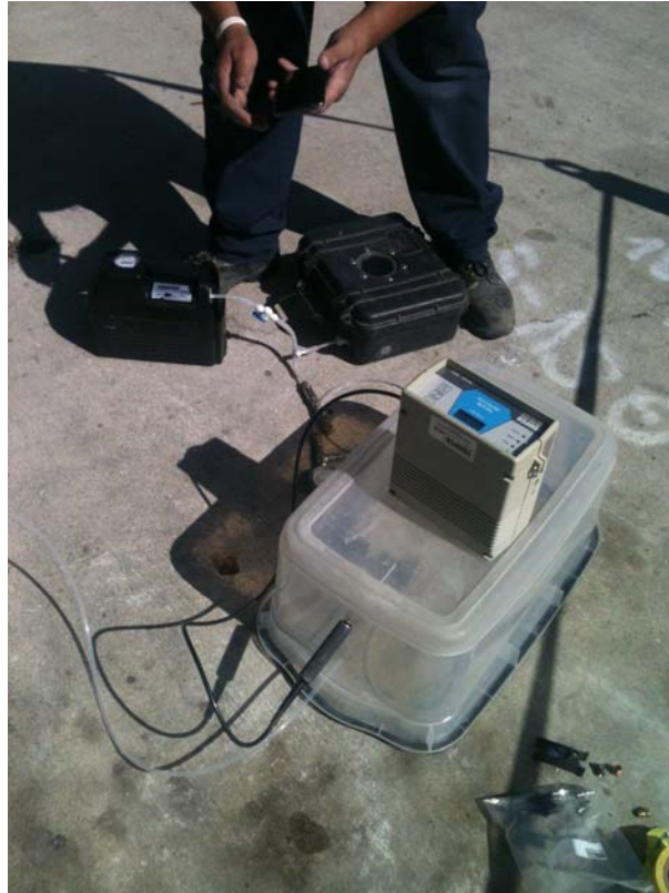
Plate 31. Soil vapor sample set up on SV-5
