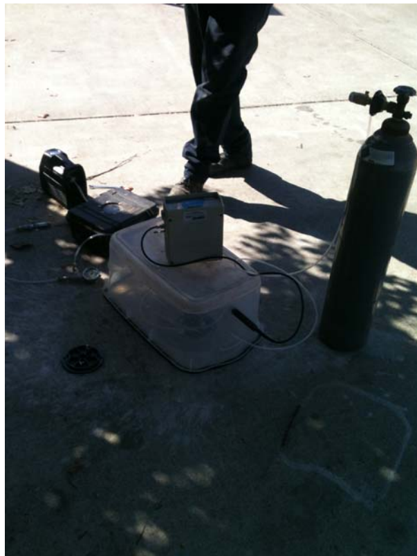
Plate 28. Soil vapor sample set up on SV-4
