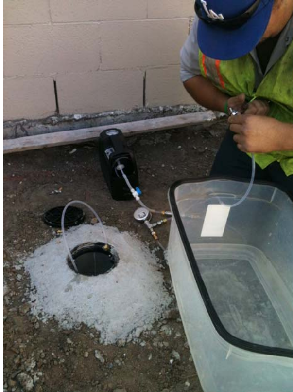
Plate 25. Vironex setting up to sample soil vapor at SV-2
