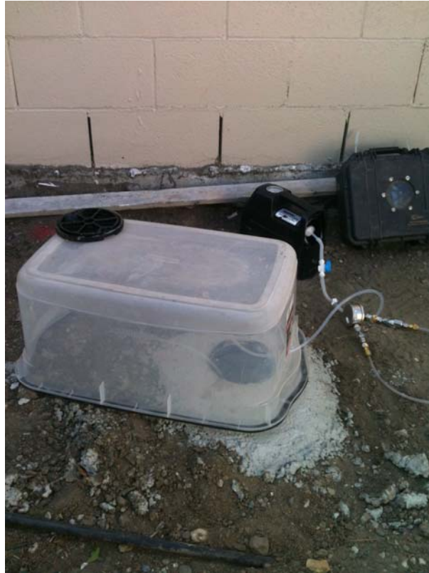
Plate 27. Soil vapor sample set-up on SV-2
