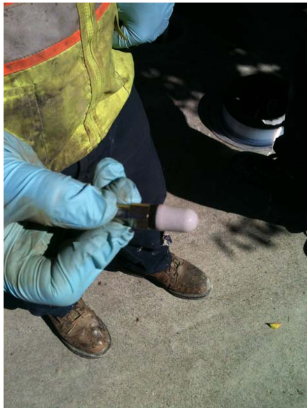
Plate 6. Vapor sampling tip used to construct vapor points
