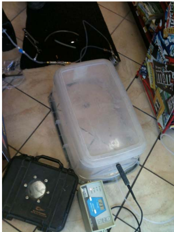
Plate 34. Soil vapor sample set up on SSG-2
