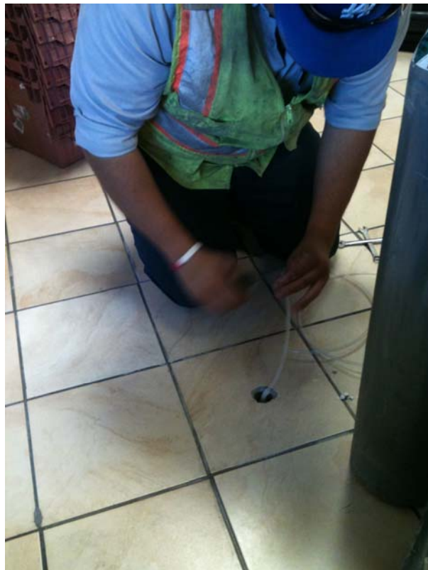
Plate 36. Vironex setting up for soil vapor sampling
