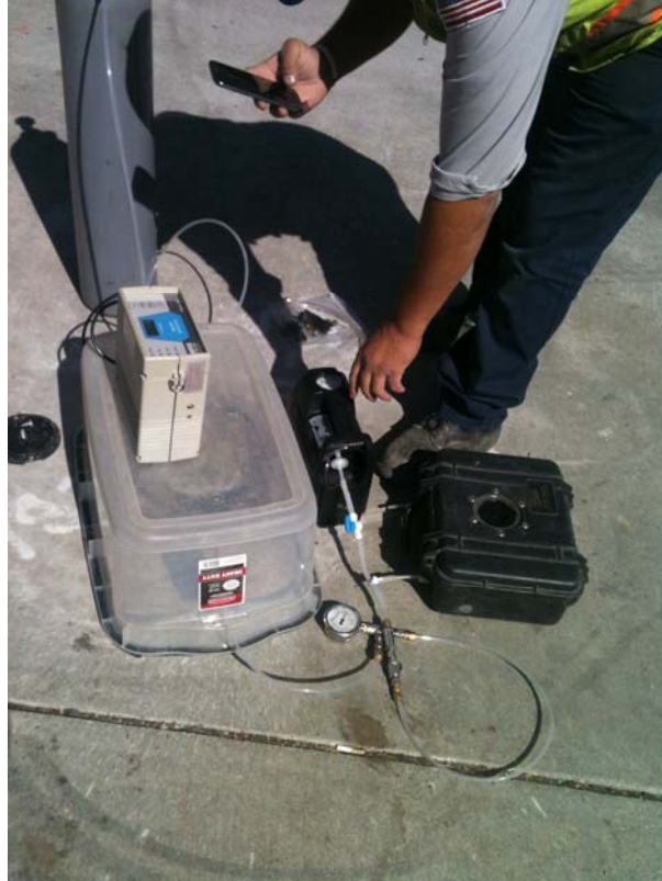
Plate 29. Soil vapor sample set up on SV-3
