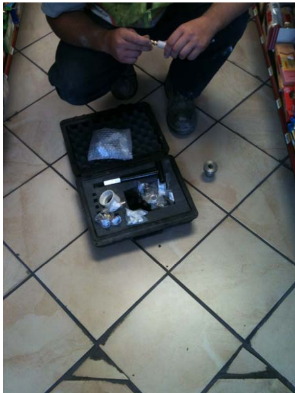
Plate 20. Prepping to install indoor soil vapor sampling pins
