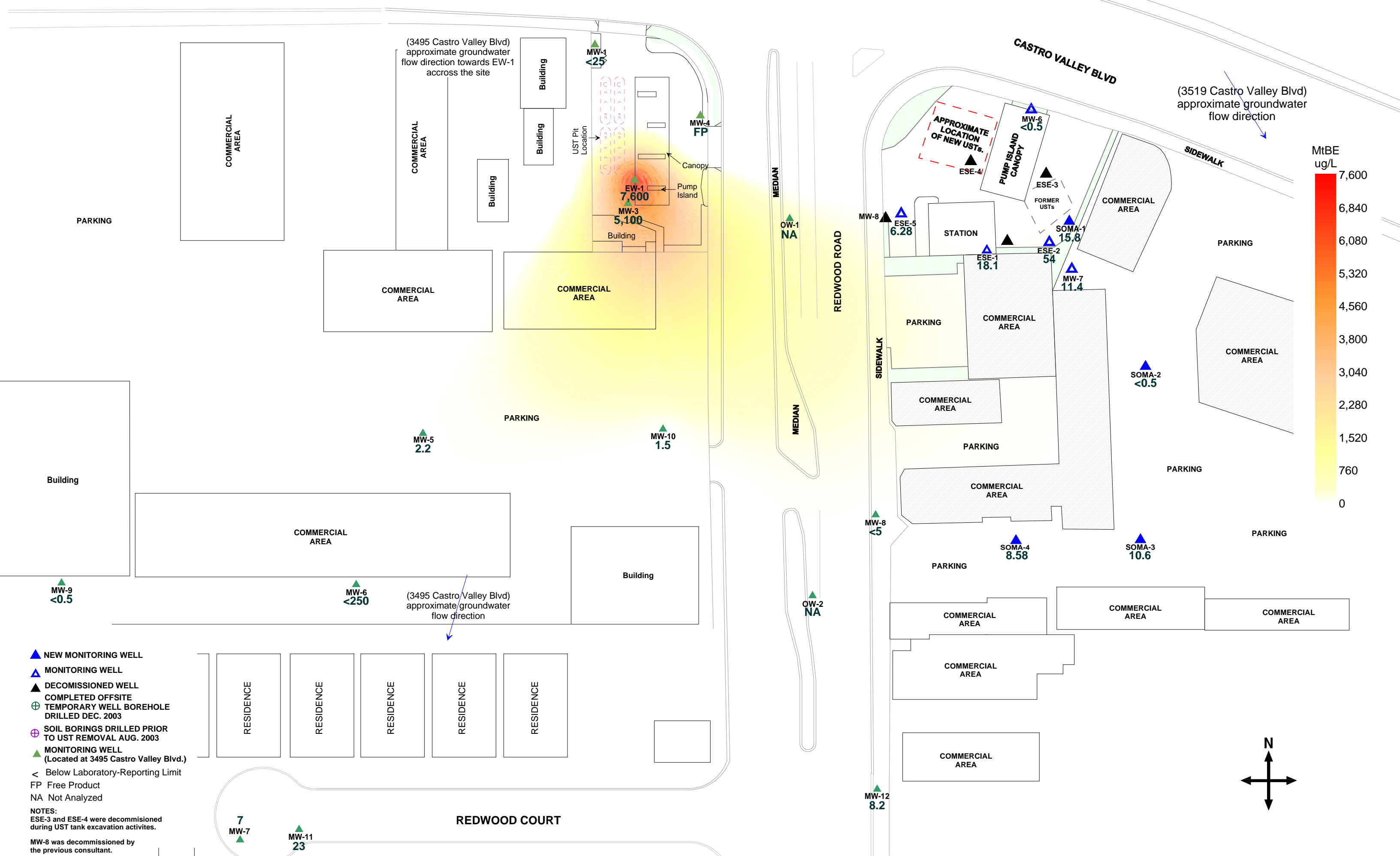
Figure 5: Contour Map of MtBE Concentrations (EPA Method 8260B) in Groundwater July 16, 2008
