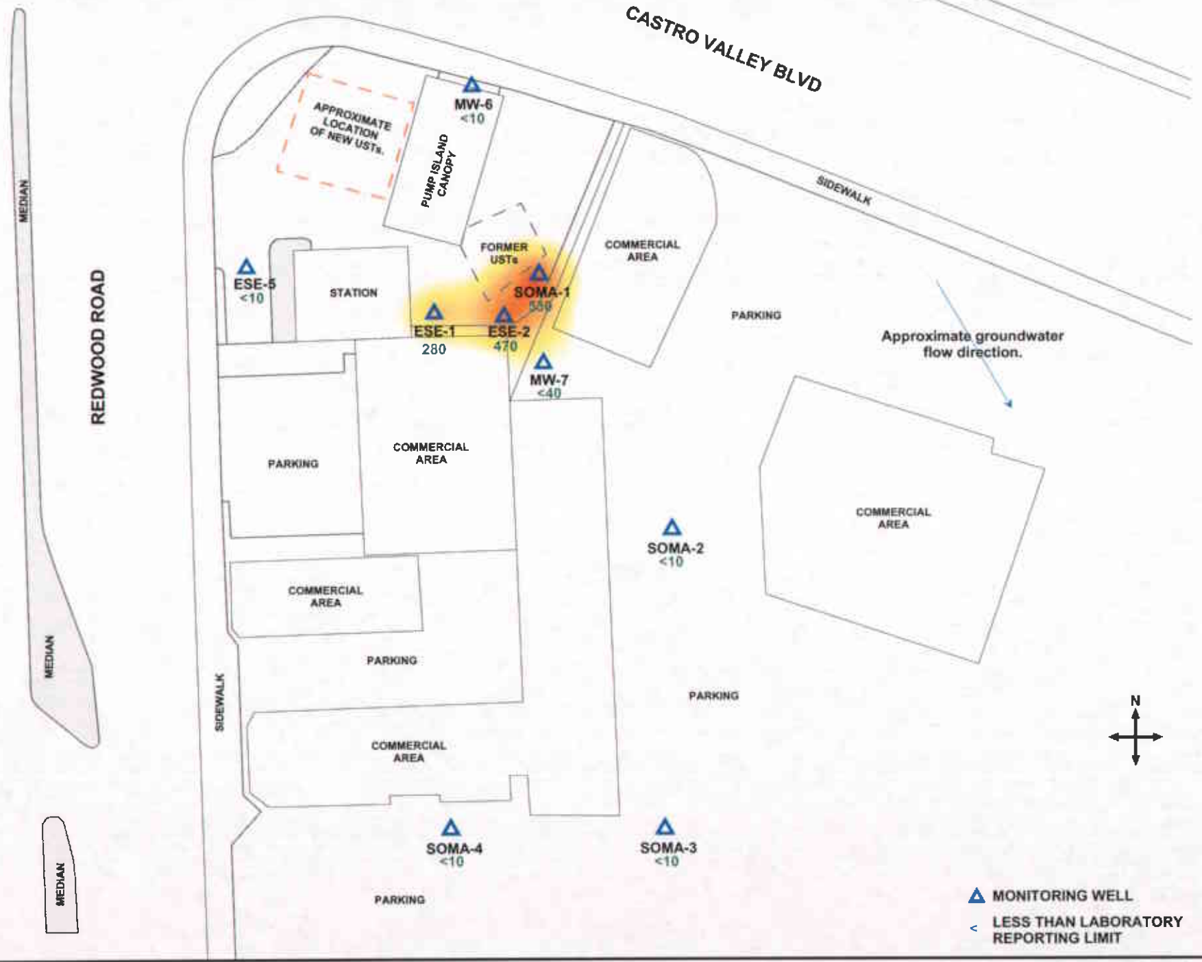
Figure 7: Contour map of TBA concentrations in groundwater, January 2005.
