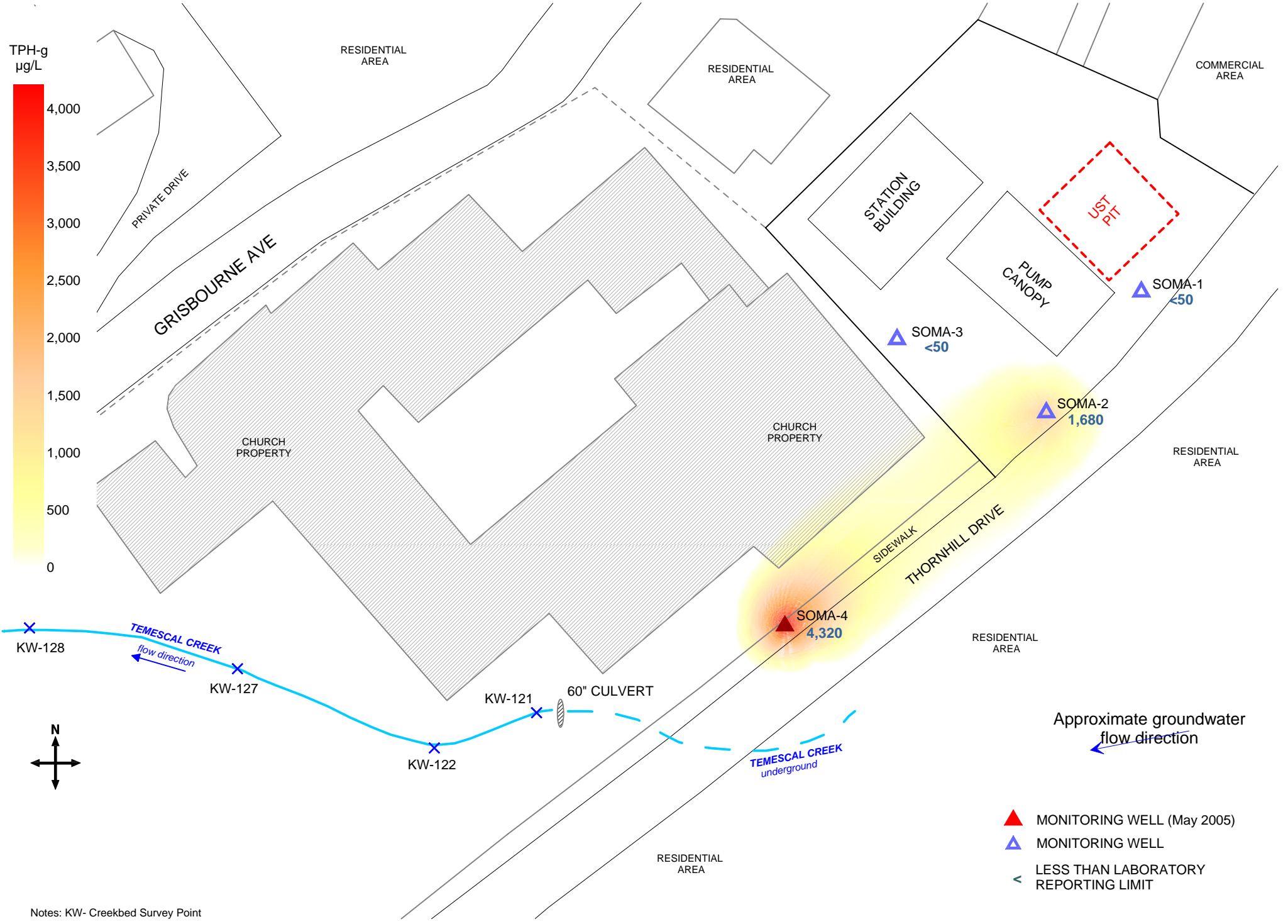
Figure 4: Contour map of TPH-g concentrations in groundwater. October 30, 2006.
