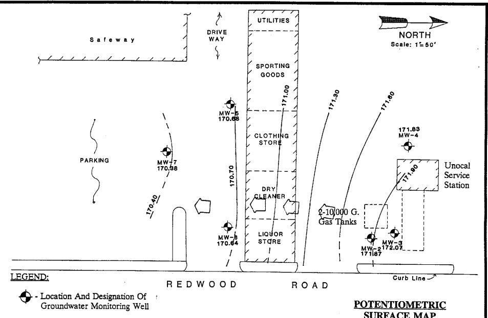
Line Of Equal Potentiometric Surface Elevation (10/08/92)
