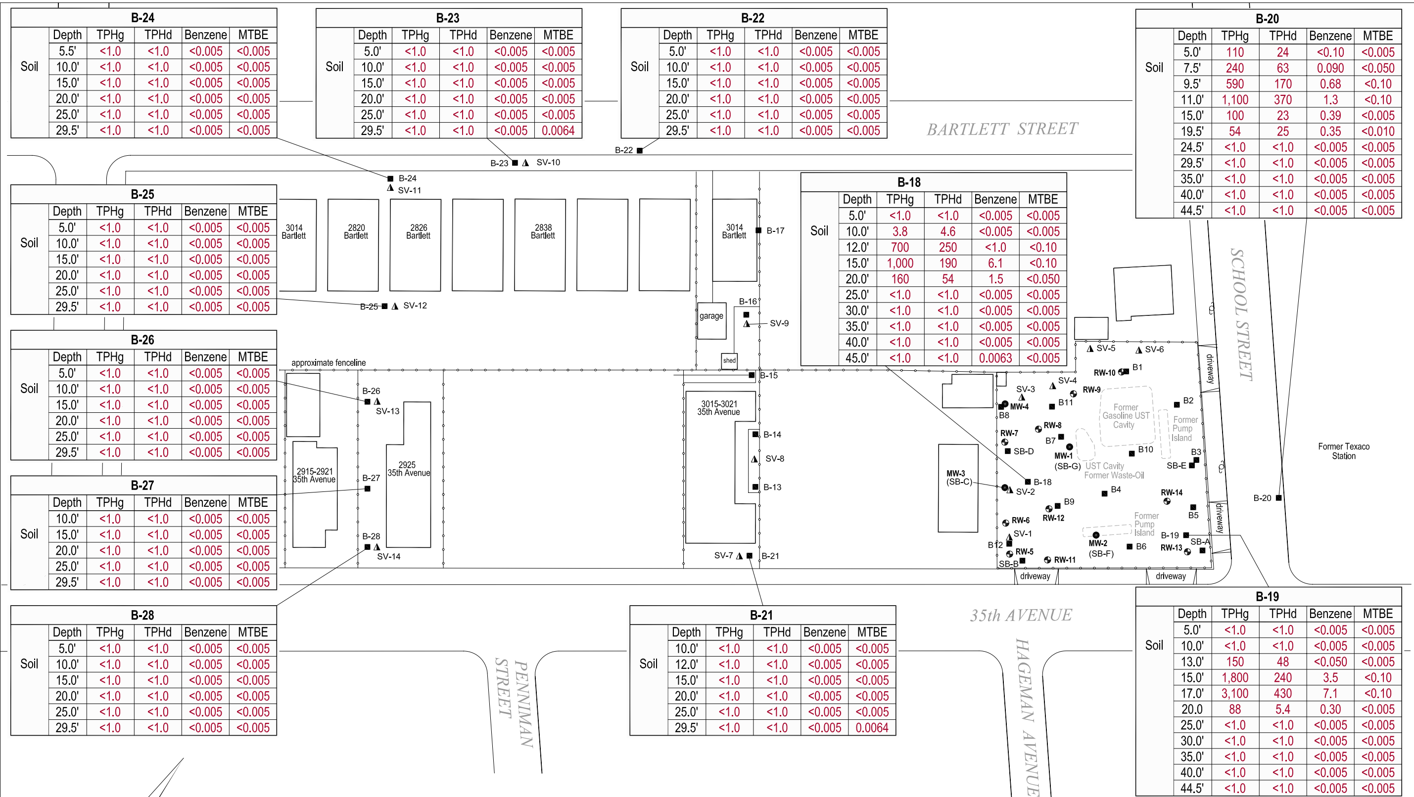
FIGURE 7 PHASE II HYDROCARBON CONCENTRATIONS in SOIL FORMER EXXON STATION 3055 35th AVENUE Oakland, California
