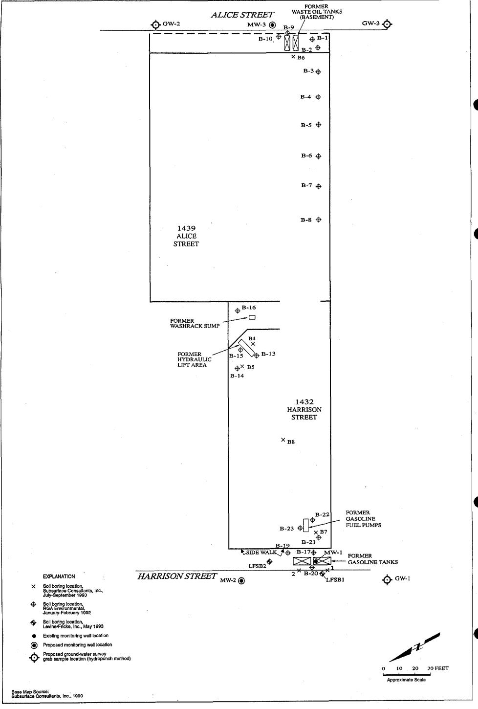
Figure 1: SITE PLAN SHOWING PROPOSED MONITORING WELLS AND GROUND-WATER SURVEY GRAB SAMPLING LOCATIONS
