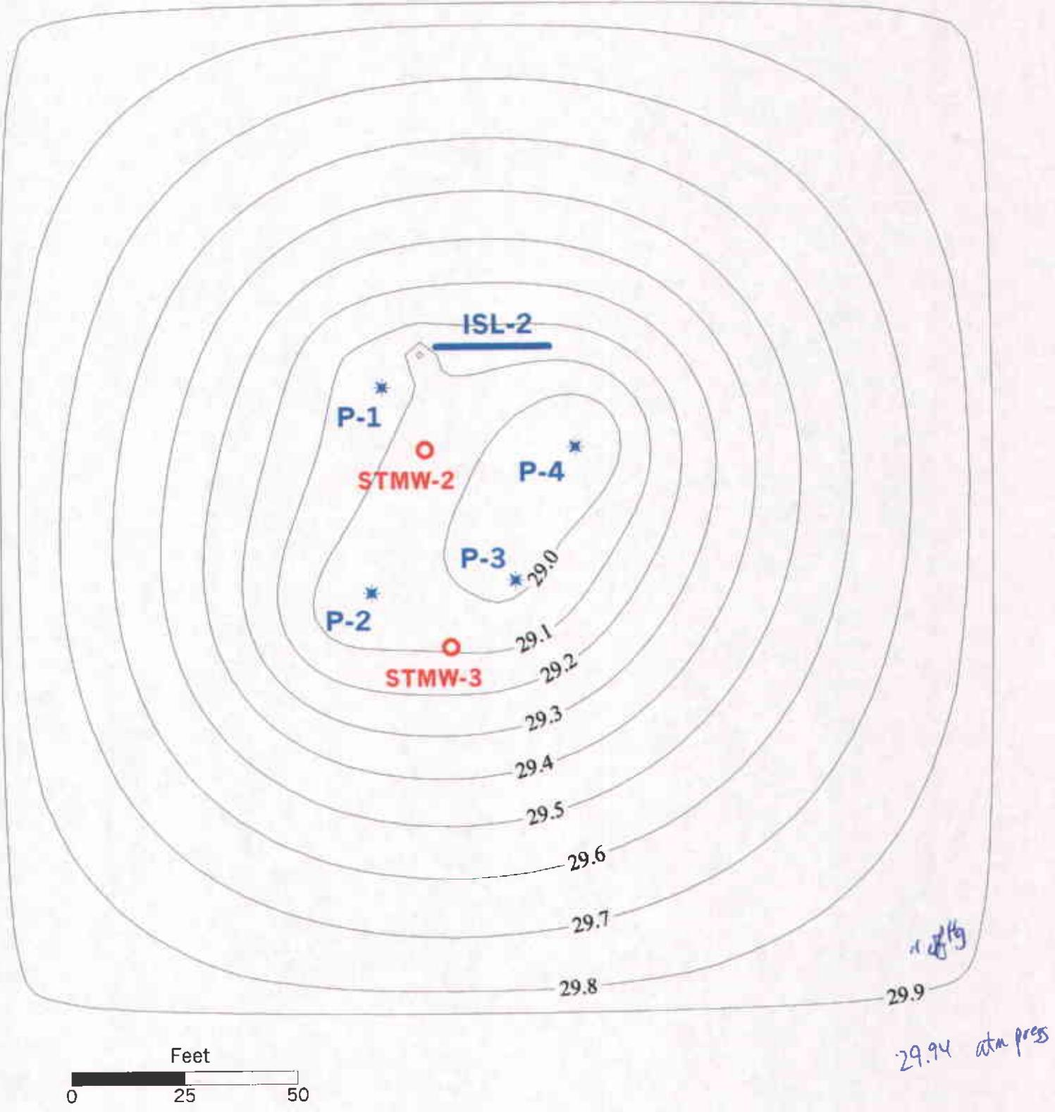
Figure 3: Simulated Pressure Contours around Vapor Extraction Wells
