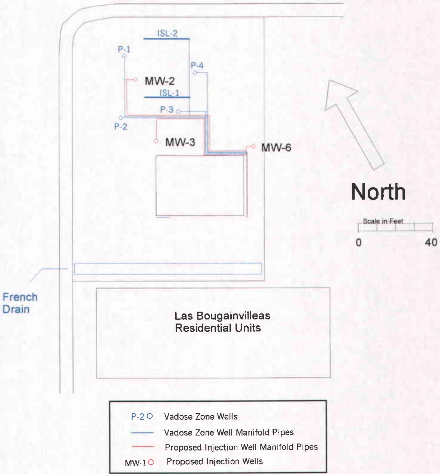
Figure 2: Location of Vapor Extraction Wells
