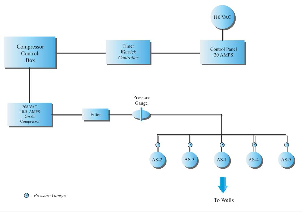
Figure 10: Block diagram of the Air Sparge System
