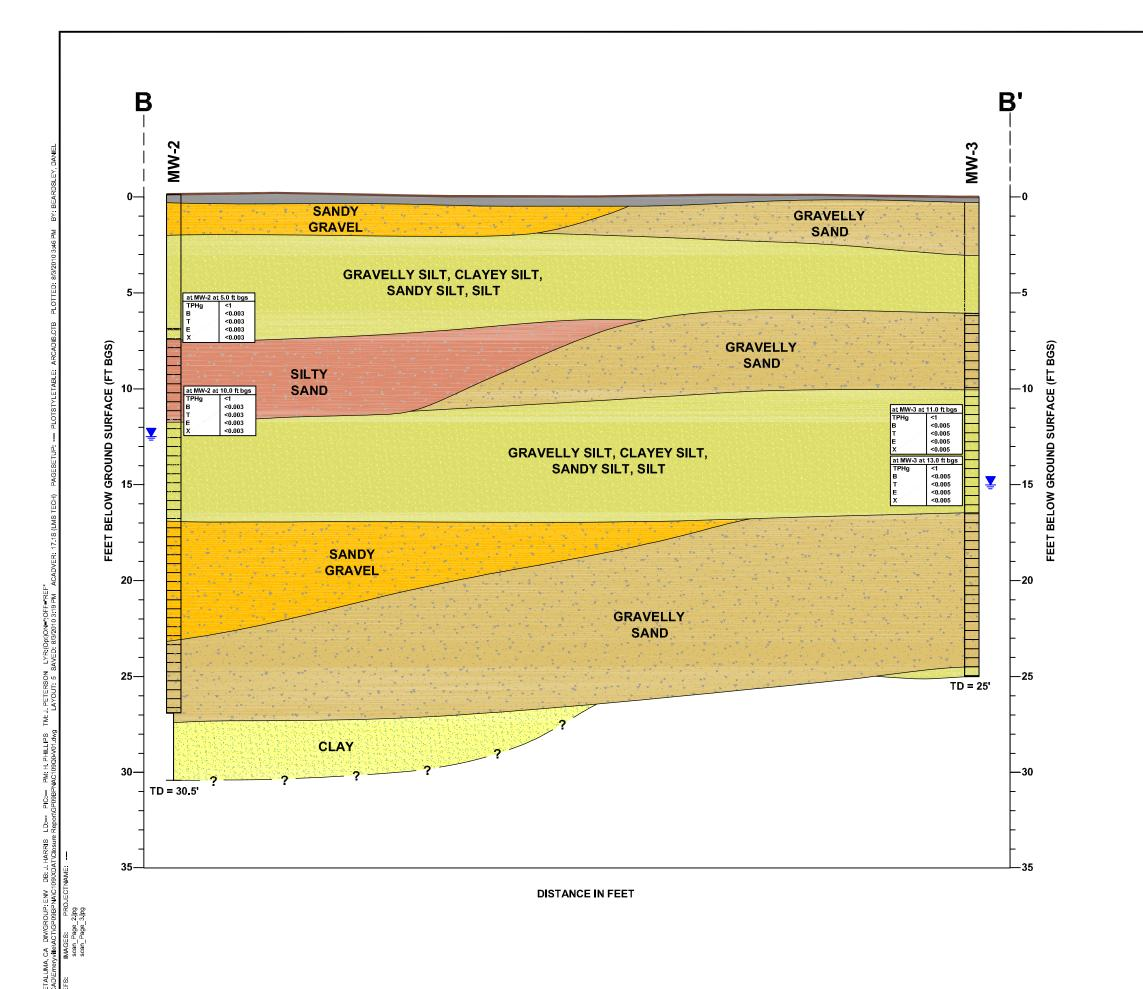
LEGEND CLAY (CH) GRAVELLY SILT, CLAYEY SILT, SANDY SILT, SILT (ML) SILTY SAND (SW) GRAVELLY SAND (SW) SANDY GRAVEL (GW) ASPHALT —?— CONTACT INFERRED WELL SCREEN TD TOTAL DEPTH WATER LEVEL DURRING DRILLING TOTAL PETROLEUM HYDROCARBONS AS GASOLINE BENZENE TOLUENE ETHYLBENZENE XYLENE
