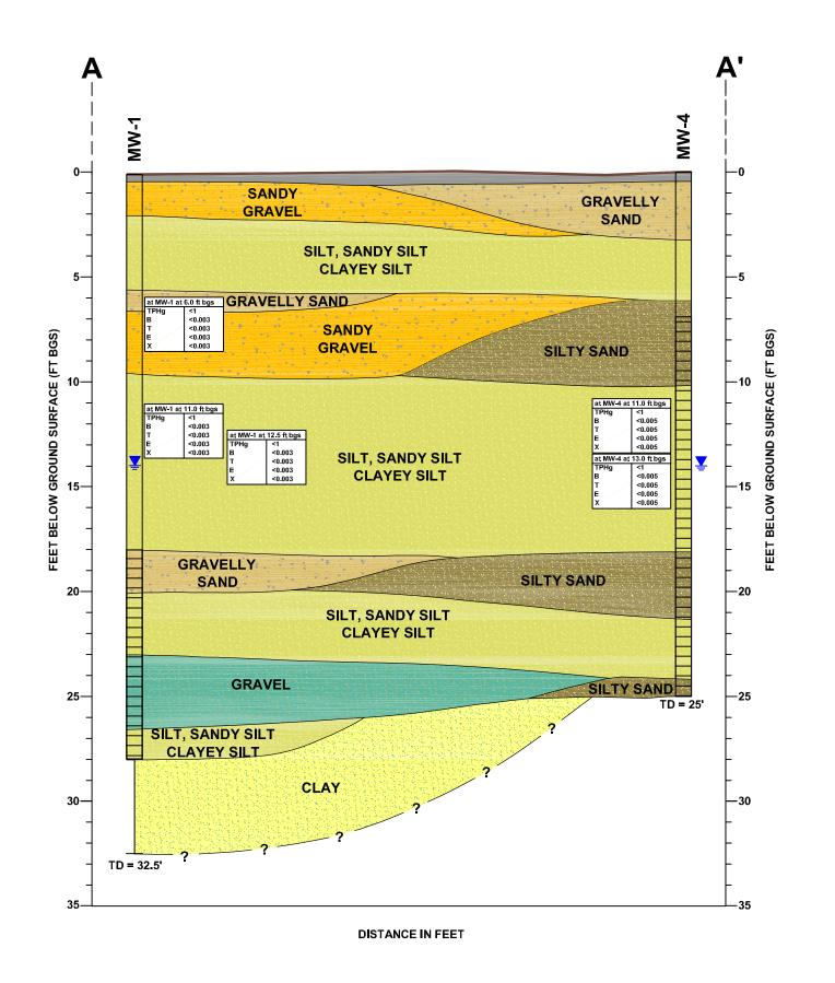
LEGEND CLAY (CH) SILT, SANDY SILT, CLAYEY SILT (ML) SILTY SAND (SM) GRAVELLY SAND (SW) SANDY GRAVEL (GW) GRAVEL (GP) ASPHALT —?— CONTACT INFERRED WELL SCREEN TOTAL DEPTH TD WATER LEVEL DURRING DRILLING TOTAL PETROLEUM HYDROCARBONS AS GASOLINE BENZENE TOLUENE ETHYLBENZENE XYLENE
