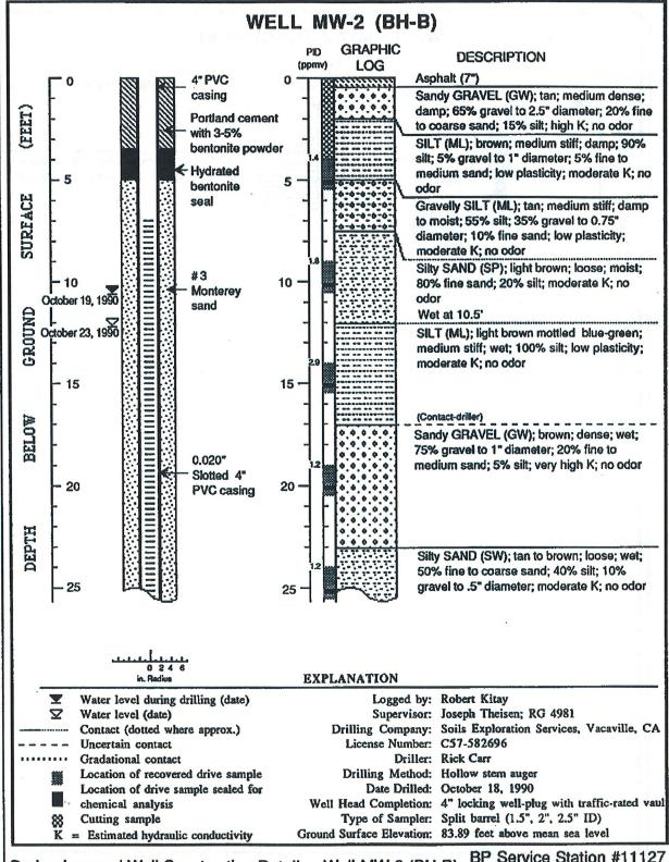
Boring Log and Well Construction Details - Well MW-2 (BH-B)
