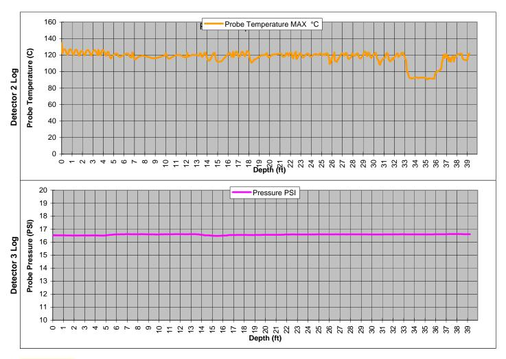
Explanation: Pre drill to 3' bgs. Hand auger to 5' bgs. No conductivity - GREGG CPT. Refusal at 39.2' bgs.
