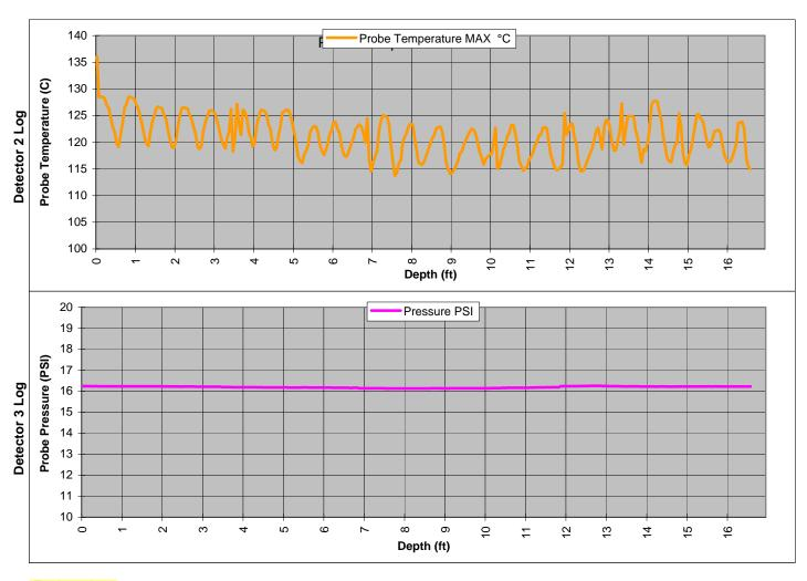
Explanation: Pre drill to 3' bgs. Hand auger to 5' bgs. No conductivity - GREGG CPT. New membrane.
