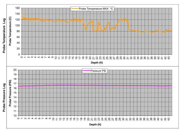
Explanation: Pre drill to 3' bgs. Hand auger to 5' bgs. No conductivity - GREGG CPT. Refusal at 43.75' bgs.
