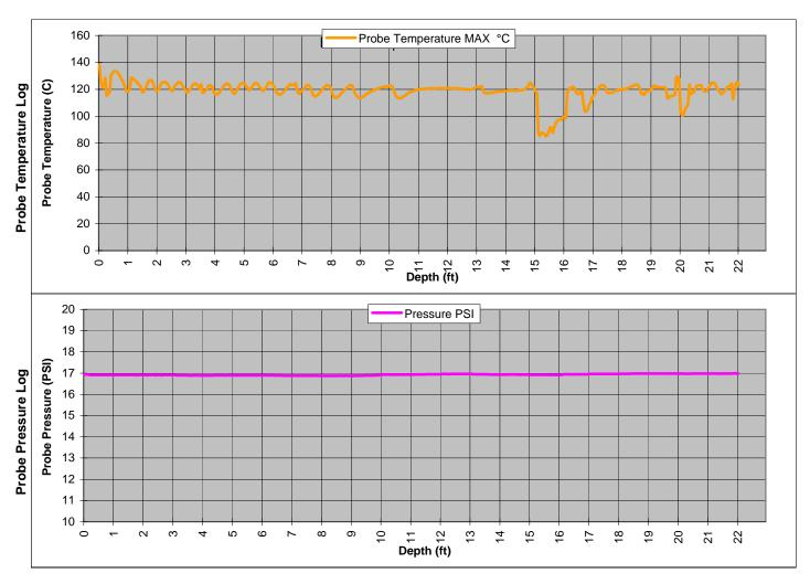
Explanation: Pre drill to 3' bgs. No conductivity - GREGG CPT. Refusal at 22' bgs.
